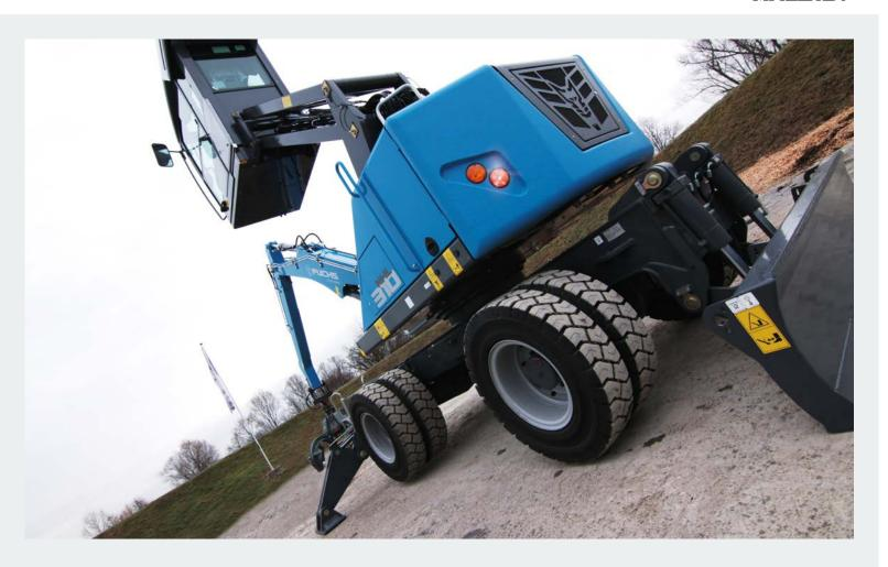
Transport position with dozer blade; undercarriage rotated by 180°
