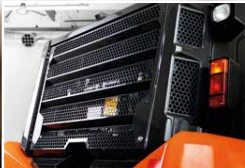
New rear grill protects radiator compartment.
