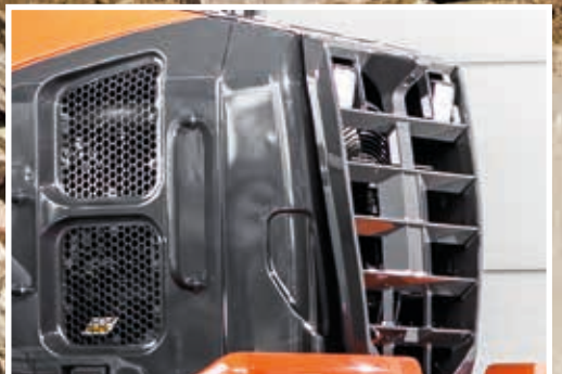
Anti-clogging radiators enhance durability.
