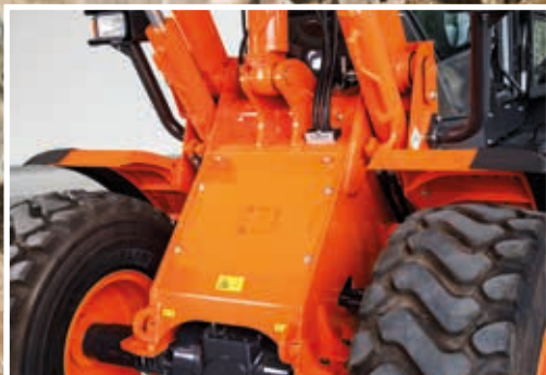
The front frame of the ZW150-6 has been reinforced.
