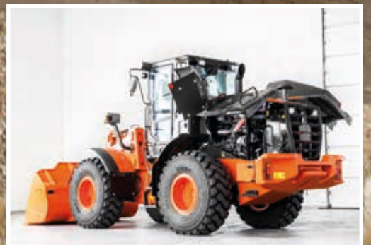
Easy access for maintenance from ground level.
