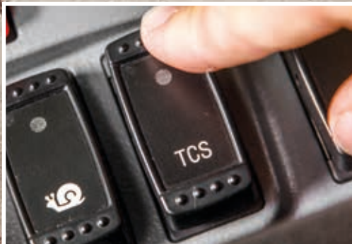
The traction control system helps to avoid tyre slippage in wet or wintry conditions.
